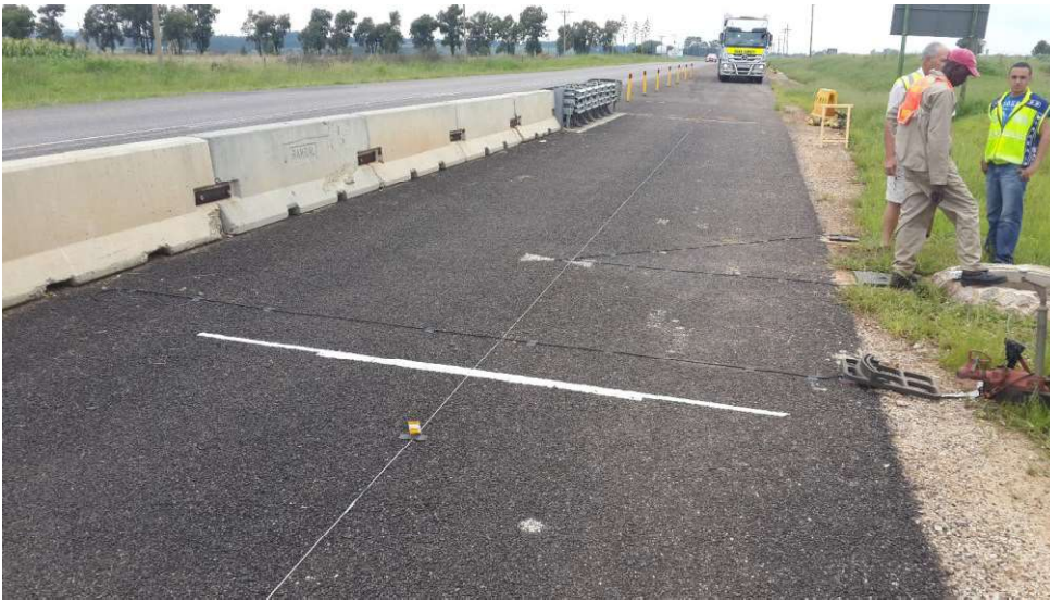
Figure 5.1: Example of the use of traffic-counter tubes to determine wheel wander in South Africa.
