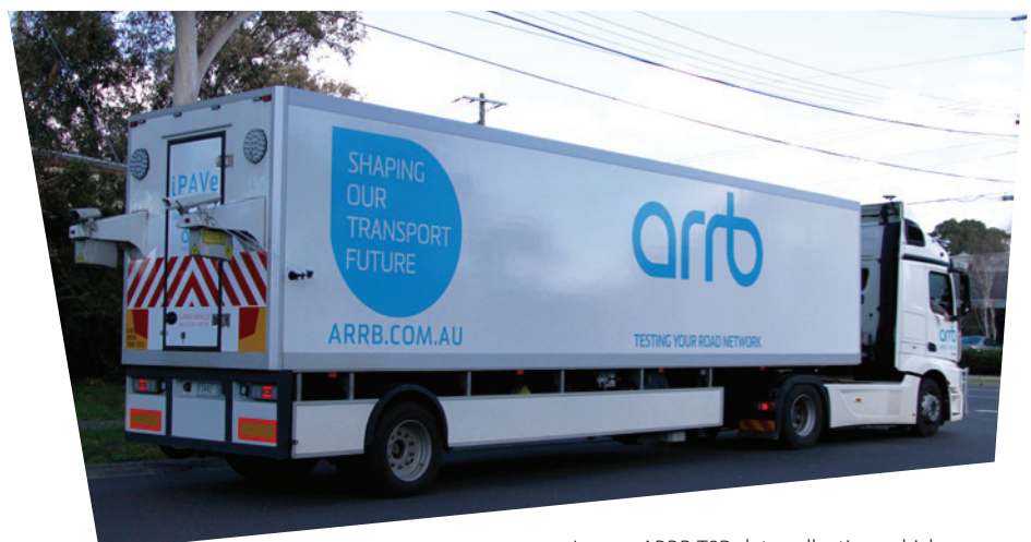
Image: ARRB TSD data collection vehicle Source: ARRB (2021)
