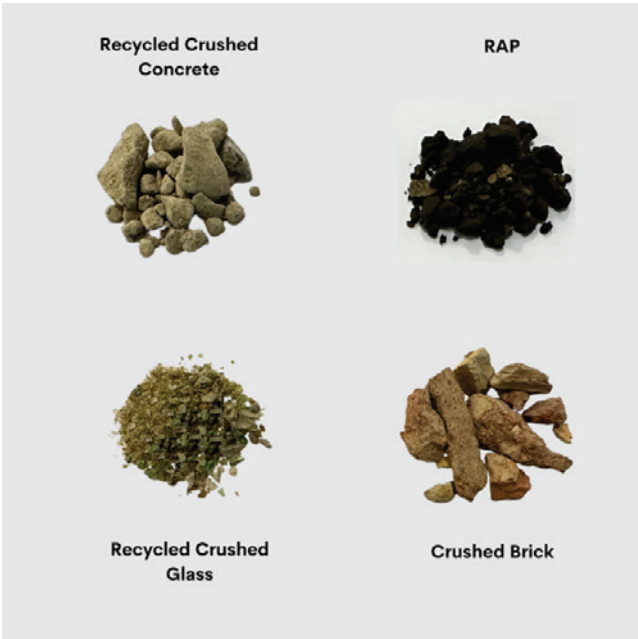
Image: Recycled materials tested in the lab Source: ARRB (2022)
