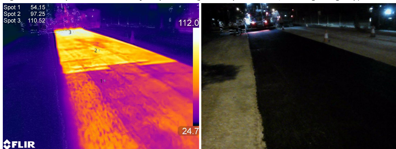
Figure 4.15: Temperature measured by temp. camera (just after paver moved, following a long stop)
