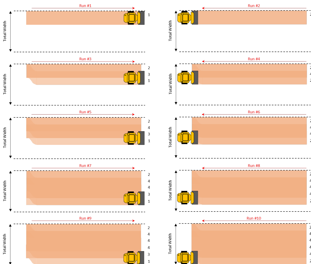
Figure 4.9: Rolling pattern and need for extra pass to achieve target number of passes
