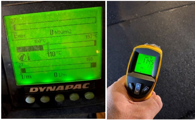
Figure 2.29: Verification process of mounted temperature sensors
