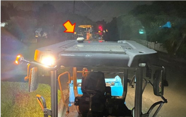
Figure 2.19: Position of the GPS antenna
