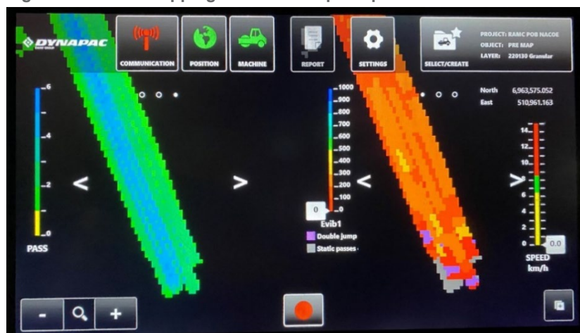
Figure 3.2: Pre-mapping before the asphalt placement
