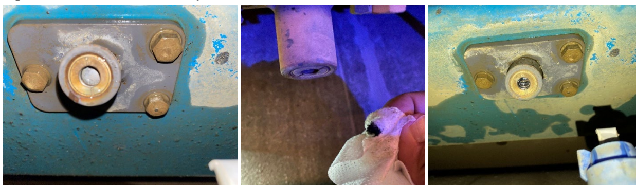
Figure 2.28: Maintenance of temperature sensors
