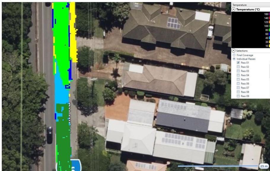
Figure 4.16: IC temperature data, recorded at the same location – Pass #1
