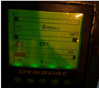
Figure 2.8: Display showing basic IC measured attributes
