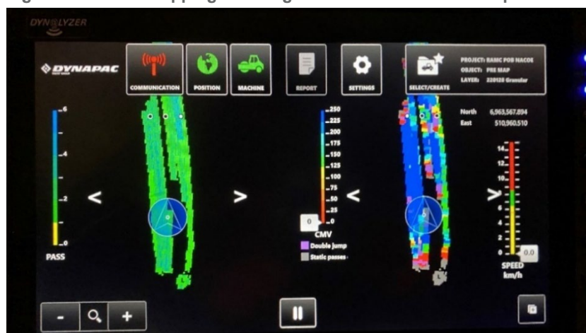
Figure 3.3: Pre-mapping – finding the weak areas and soft spots
