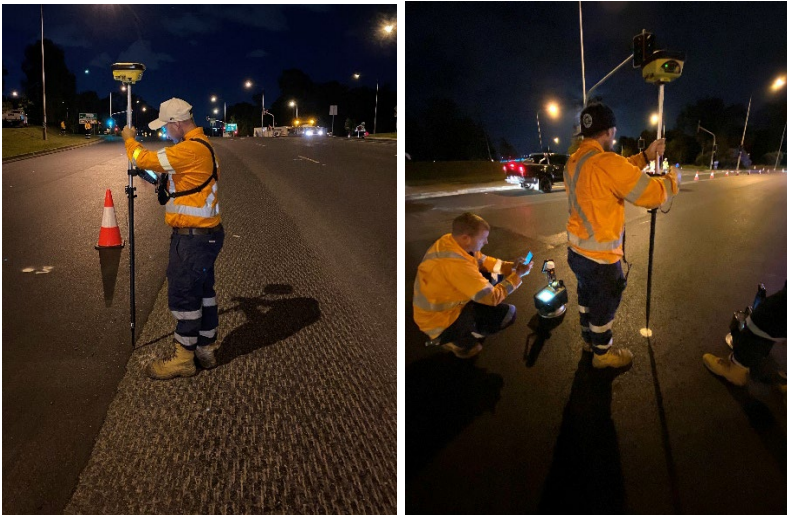
Figure 3.7: Using the rover for recording the coordinates of test spots and boundaries
