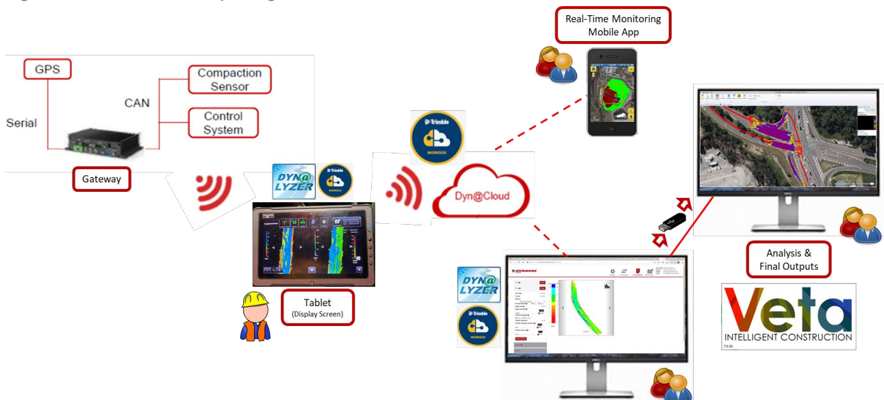
Figure 2.30: Data flow and packages used for IC
