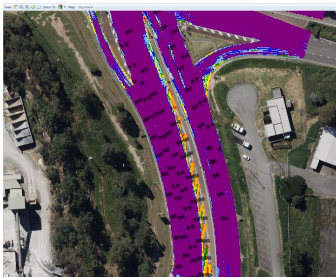
Figure 4.23: PQI test results on the wearing course (including locations) in Veta
